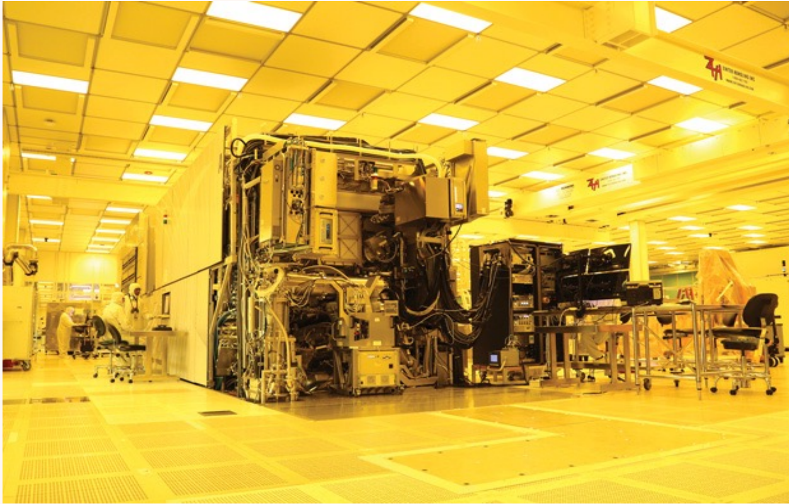
EUV scanner ASML NXE:3300B > 100 M$ 1.5 MWatt SUNY Polytechnic Institute, Albany, NY
